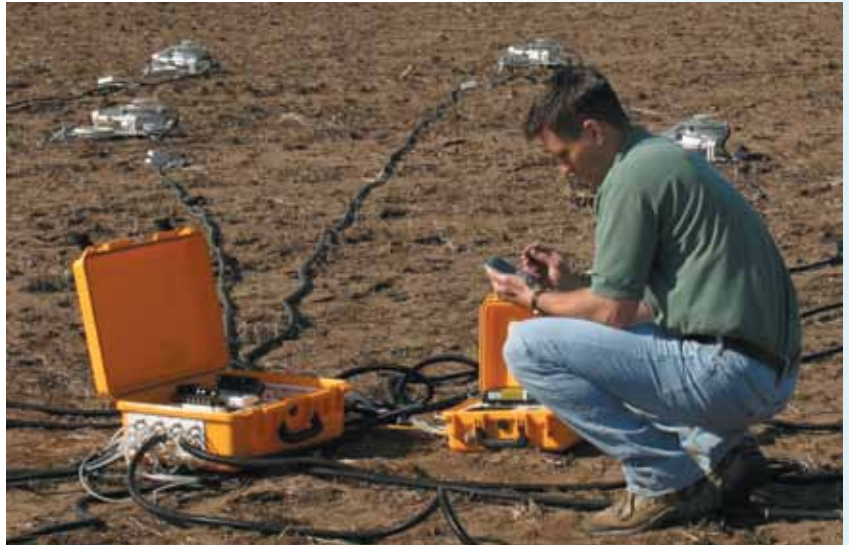
LI-8150 Multiplexer (left), four long-term chambers (background), LI-8100A Analyzer Control Unit (right), communication through wireless PDA.
