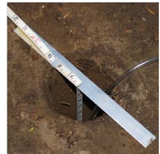
Fig. 19. Tape secured using Tape Holder.
