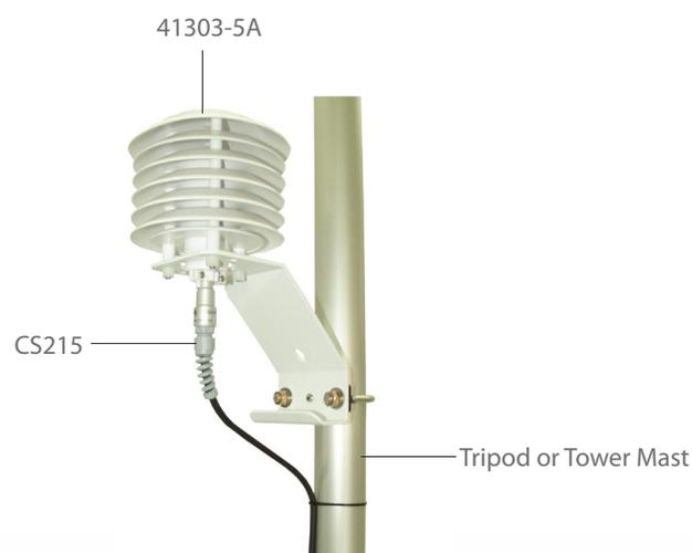
Above is a sensor housed in the 41303-5A radiation shield. The U-bolt is placed in the holes on the side of the bracket to allow the 41303-5A to be attached to a mast or vertical pole.
