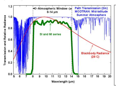
Spectral response of SI series infrared radiometers. Spectral response (green line) is determined by the germanium filter and corresponds closely to the atmospheric window of 8-14 μm, minimizing interference from atmospheric absorption/emission bands (blue line) below 8 μm and above 14 μm. Typical terrestrial surfaces have temperatures that yield maximum radiation emission within the atmospheric window, as shown by the blackbody curve for a radiator at 28 C (red line).
