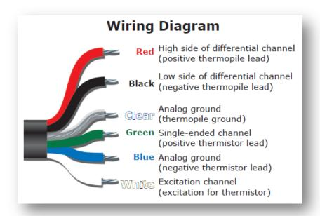
All Apogee analog infrared radiometer models (SI-100 series) have sensor-specific calibration coefficients determined during the custom calibration process. Unique coefficients for each sensor are provided on a coefficient certificate (shown on following page).
