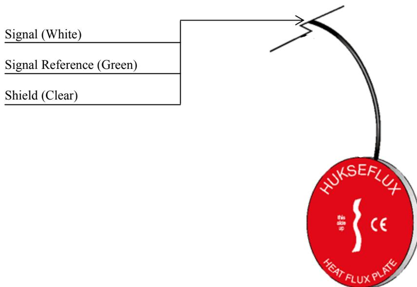
FIGURE 6-2. HFP01 plate to datalogger connections
