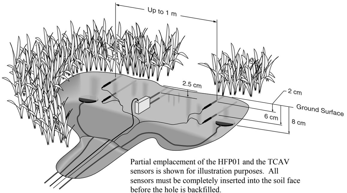
FIGURE 6-1. Placement of heat flux plates
