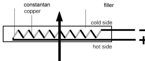
FIGURE A-1. General characteristics of a heat flux sensor
