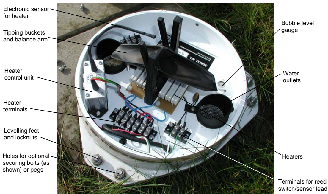
Figure 4 Internal View of SBS500H (Heated Version)
