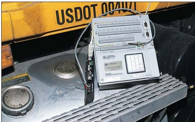
Left of the CR5000 datalogger is a SDM-CAN. It allows a vehicle's on-board diagnostic system to output standardized data streams that are synchronized with other measurements and stored in the CR5000.
