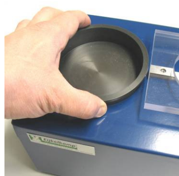
Fig. 10: Removing soil container from apparatus.
