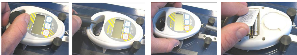
1. Unscrew 2. Remove screw 3. Remove balance 4. Remove 2x AAA batteries. Fig. 17: Steps for replacing batteries.
