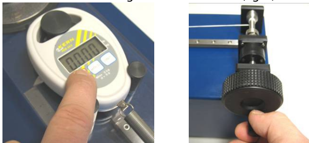
Fig. 8: Tare the scale / start winding smoothly clockwise / read the maximum value after minor movement.
