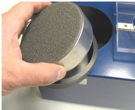
Fig. 11: Placement of sample-ring into soil container.
