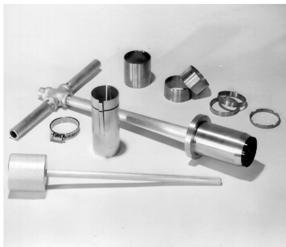
Fig. 1c Soil Core Sampler (Model 0200) shown with various sizes of brass cylinders for obtaining undisturbed soil cores.
