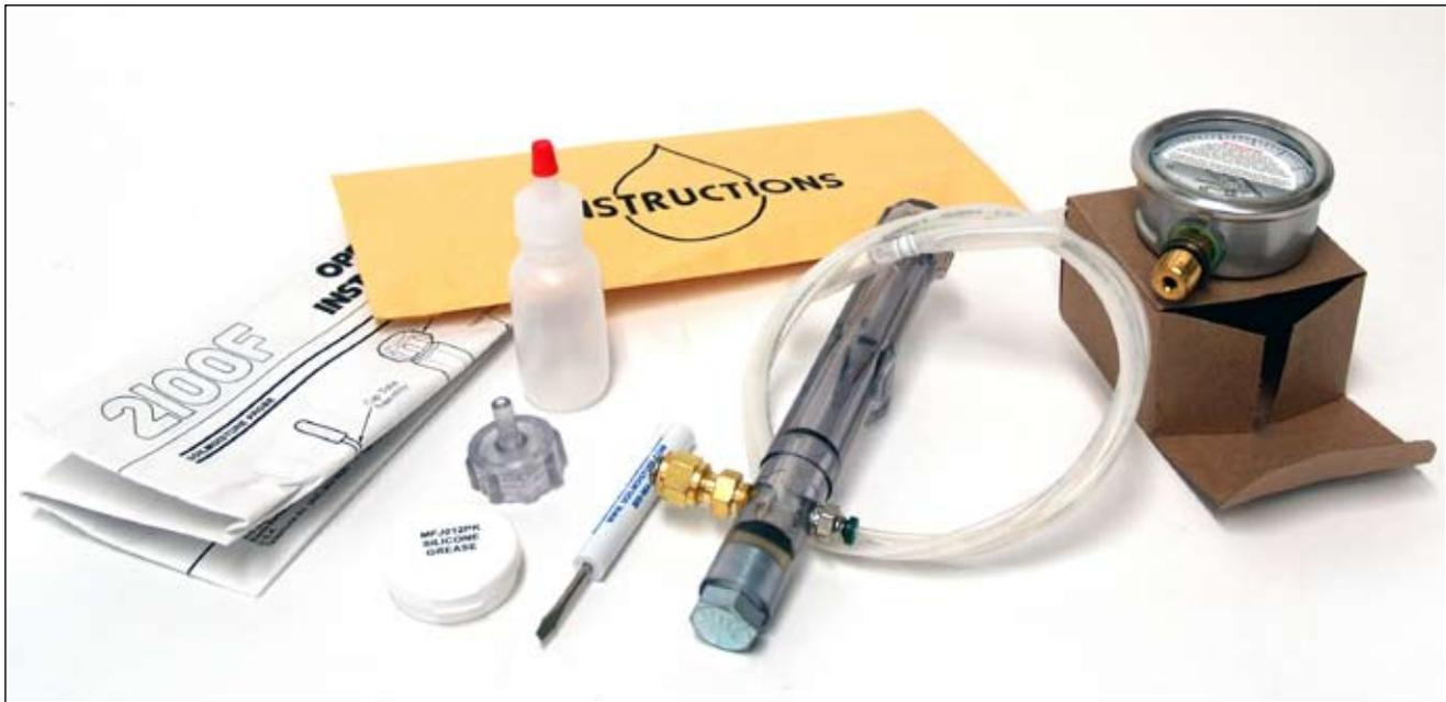
(Figure 1) - 2100F Soilmoisture Probe Kit
