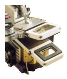
Illuminating the bottom of a leaf is particularly useful for survey and erect foliage measurements. The Clear Chamber Bottom has a Propafilm® window similar to the standard chamber top. Leaf temperature is computed using energy balance by measuring with a small thermocouple the temperature of air exiting the chamber.
