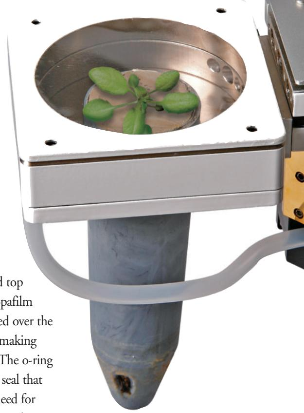
An o-ring sealed top plate with a Propafilm covering is placed over the chamber when making measurements. The o-ring provides a tight seal that eliminates the need for traditional foam gaskets.
