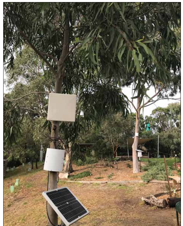
Figure of SFM1 Sap Flow Meter, Solar Panel & Antenna at CERES.
