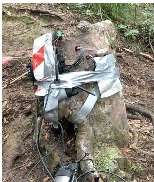
Figure (above, right) shows SFM1 Sap Flow Meters monitoring sap flow through the stump at different times of day. (Supplied by Assoc. Prof. Sebastian Leuzinger)
