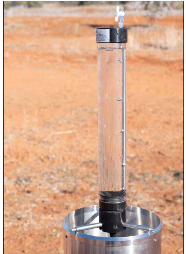
Figure of Tipping Bucket Rain Gauge Calibration Field Kit In Use on a ICT International SRGO
