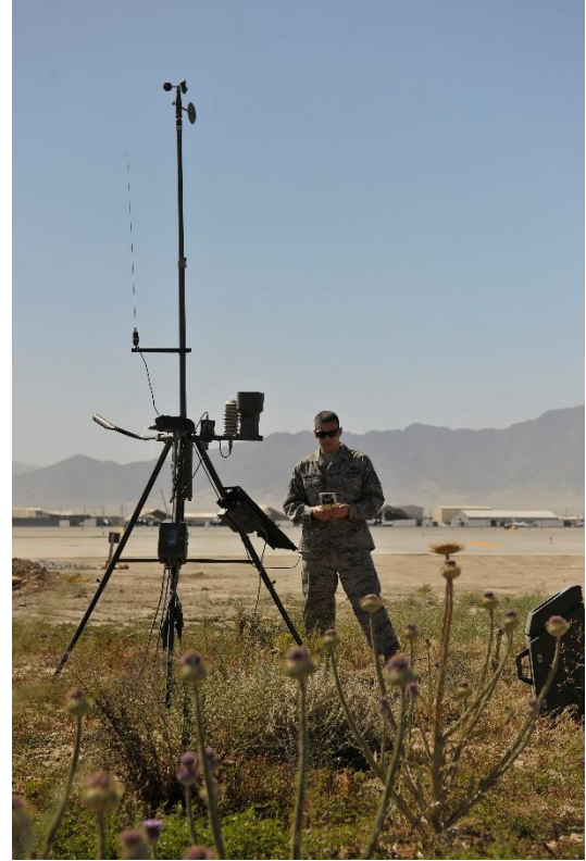
Tech. Sgt. Richard Kienzle reviews a read out from the automatic remote weather station employed by the USAF over the last 30 years. (Photo Credit: Staff Sgt. Christopher Boitz)
