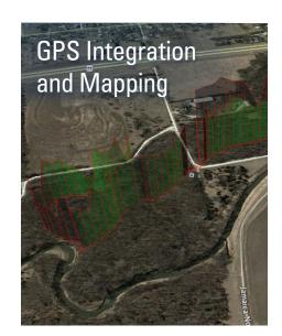
Internal GPS module integrates data into the LAI file for easy mapping in Google Earth.
