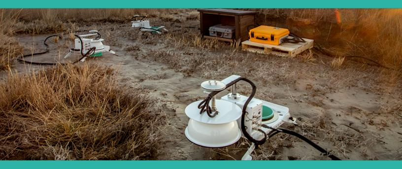
Hardware, software, and analyzers for soil gas flux research all based on extensive research and testing. Patented designs minimize disruption of natural soil gas transport across the soil surface and record high-precision flux measurements to evaluate spatial and temporal variability. The result is integrated systems that provide an ideal soil gas flux research experience. Soil gas flux systems include SoilFluxPro<sup>™</sup> Software for analysis of the dataset.
