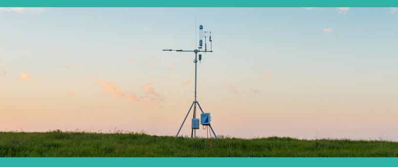
Gas analyzers feature low noise, high precision, long-term stability, and low power consumption. The SmartFlux System provides exquisite analysis of gas, wind, and biomet data, for fully processed flux results in real time. Systems include the leading eddy covariance software, including EddyPro<sup>®</sup> Software to compute results and Tovi<sup>™</sup> Software for advanced analysis of the time series.
