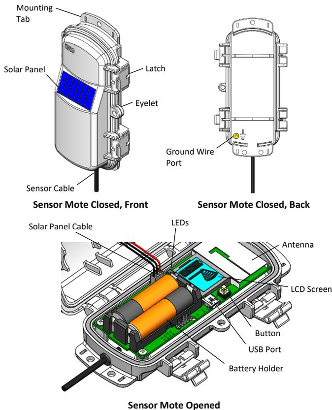
**Sensor Cable:** This is the cable that connects the mote to the sensor.
