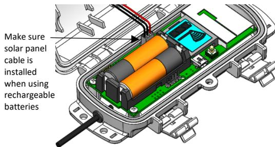
The mote contacts the network once the new batteries are installed. The green LED blinks during this process while the bars in the signal strength indicator on the LCD cycle from left to right and then the x icon blinks. Once this process is complete, the x icon is removed, the green LED stops blinking, and the blue LED begins blinking instead.
