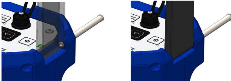
4. Push the carrying strap pin back into position using the hex key, while twisting clockwise if necessary.
