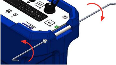
2. Remove the carrying strap pin by pressing it out of the housing chamber with the hex key. Push the pin out of the hole until it reaches the position shown.
