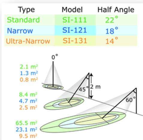
A simple FOV calculator for determining target dimensions based on infrared radiometer model, mounting height, and mounting angle, is available on the Apogee website:
