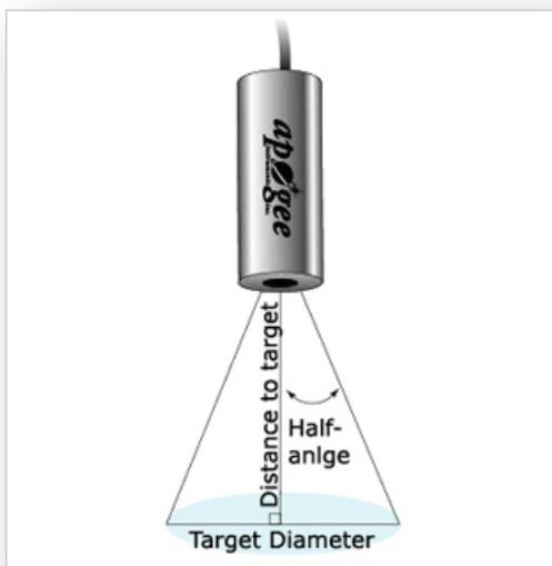
Sensor FOV, distance to target, and sensor mounting angle in relation to the target will determine target area. Different mounting geometries (distance and angle combinations) produce different target shapes and areas, as shown below.
