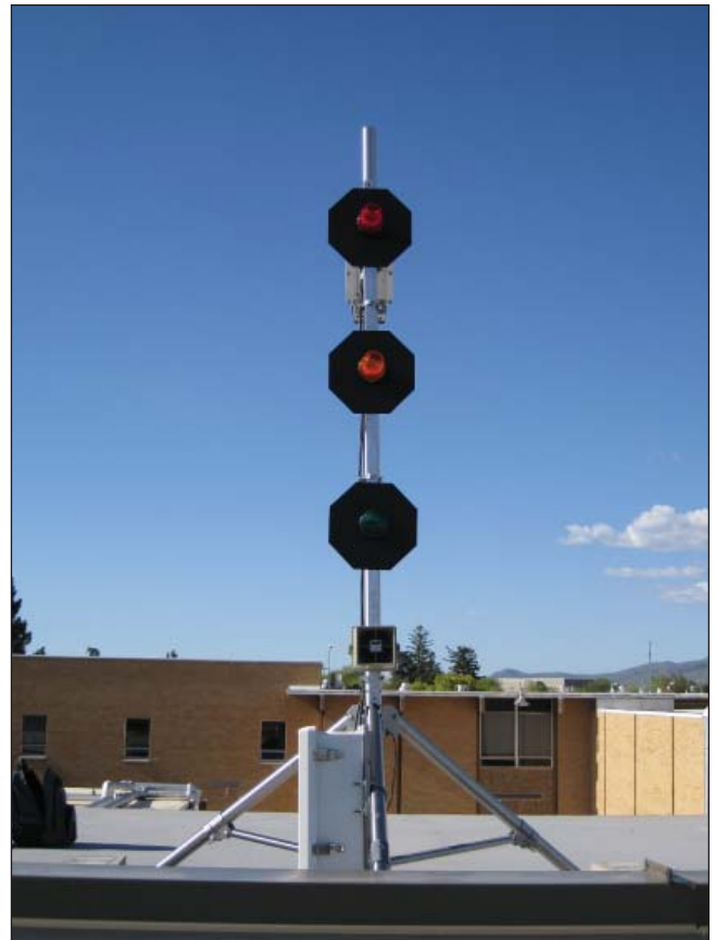
Logan High School in Logan Utah has installed a lightning warning system that includes the CS110. The CS110 is mounted to a CM110 10-ft stainless-steel tripod that sits on a roof next to the football field (left). Lights included in the system indicate the likelihood of lightning (right).
