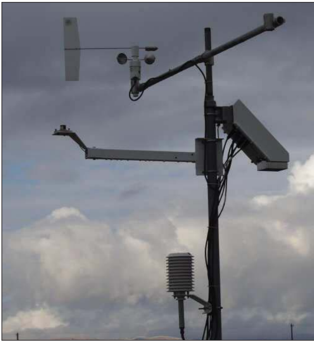
The CS110's internal datalogger can measure additional meteorological sensors—making the CS110 the center of a full weather station.
