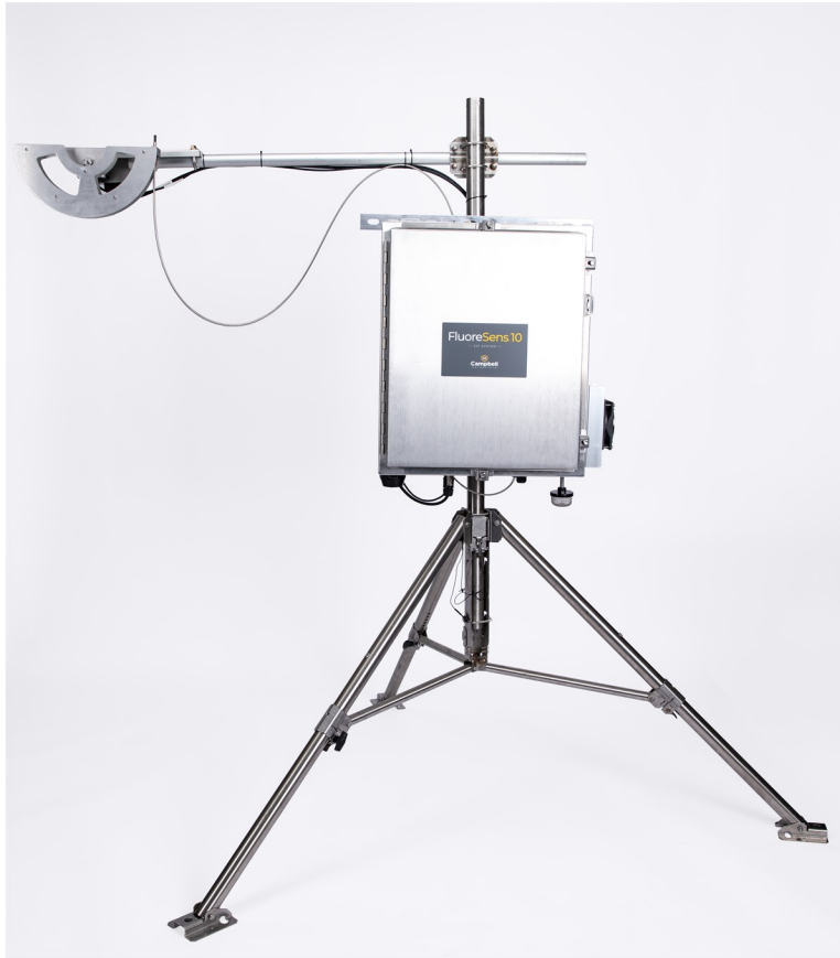
Figure 6-1. FluoreSENS 10 system mounted on a tripod (tripod and cross-arms are sold separately)
