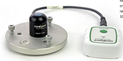
The AL-100 leveling plate is recommended for most sensors. To facilitate mounting to a cross arm, the AM-110 mounting bracket is recommended for use with the AL-100. (AL-100 leveling plate pictured)
