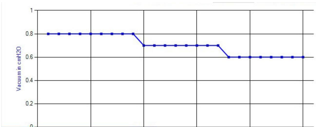
Fig. 23 - A step-like reading graph is an indication of a too short measurement time.
