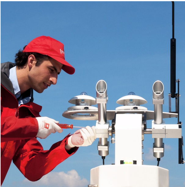
Figure 1 pyrheliometers and pyranometers on a tracker
