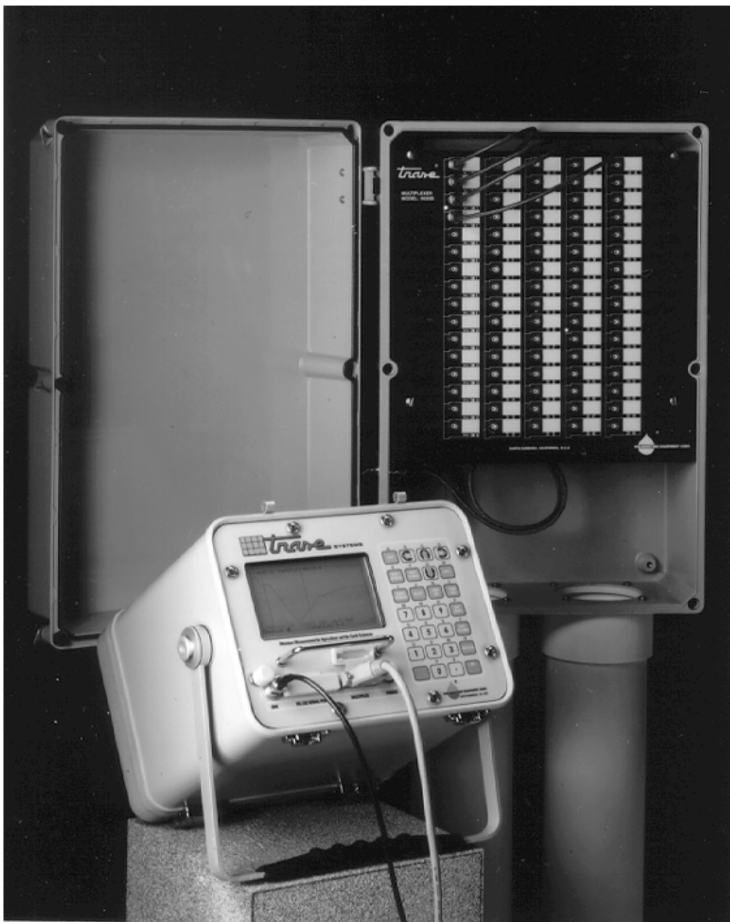
Figure 1 - Trase Unit and Multiplexer Enclosure
