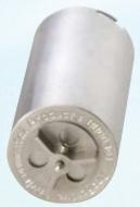
The main wear out parts consisting of the motor and seal all have been incorporated in a single replaceable motor module. Should the existing replaceable motor module fail in the field, a new replaceable motor module can quickly be installed within 60 seconds by a simple quarter turn twist!
