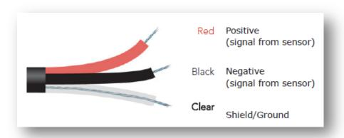
SP-230: Only apply voltage to the integrated heaters. The sensor is self-powered and applying voltage will damage the sensor.
