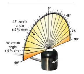
Directional, or cosine, response is defined as the measurement error at a specific angle of radiation incidence. Error for Apogee silicon-cell pyranometers is approximately  $\pm$  2 % and  $\pm$  5 % at solar zenith angles of 45° and 75°, respectively.
