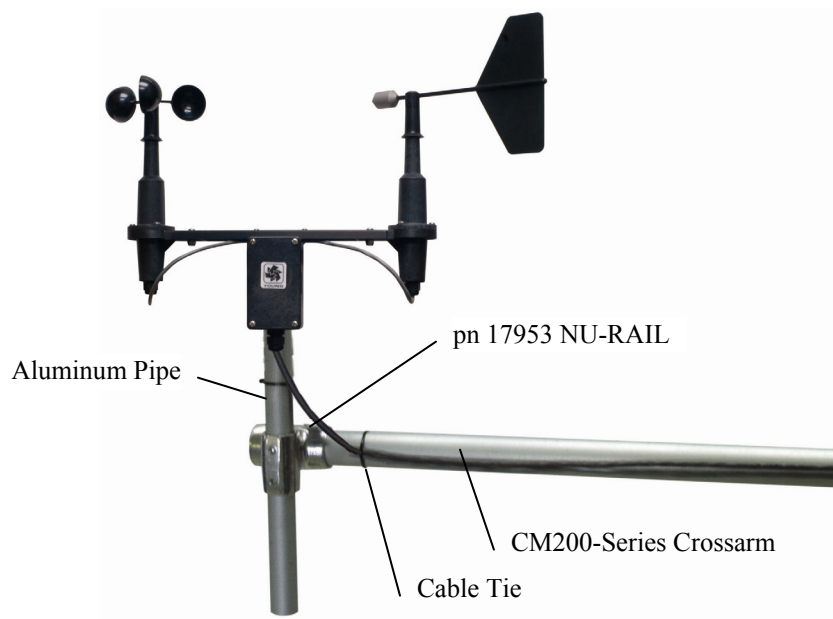
FIGURE 4-3. 03002 mounted to CM200-Series Crossarm with pn 17953
