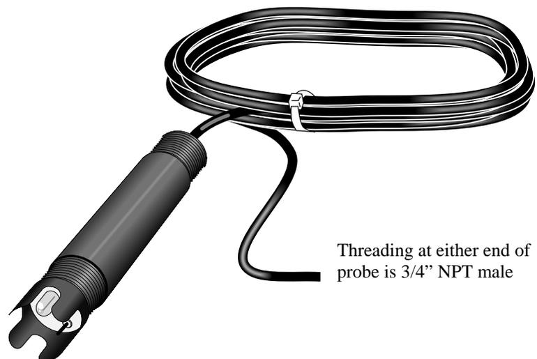
Threading at either end of probe is 3/4" NPT male
